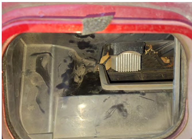
Debris on internal screen
