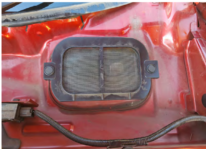
Wire Mesh fitted to Air Inlet
