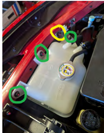
2 - NC Coolant reservoir
