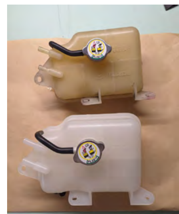
1 - NC Coolant reservoir
