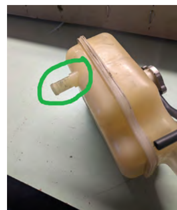
3 - NC Coolant reservoir
